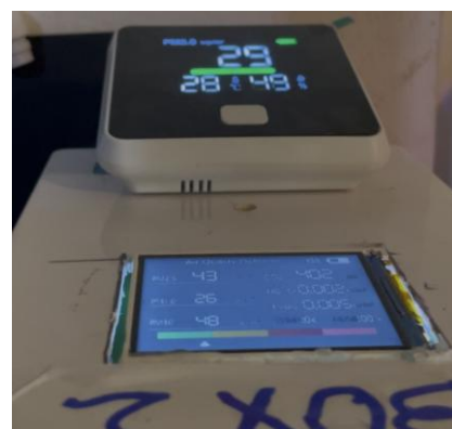
Fig. 2 Comparison of Reference and Integrated Sensors for Accuracy, Reliability and Responsiveness Testing
