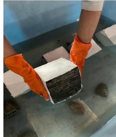
Fig. 9 Submerging testing specimens in NaCl Solution
