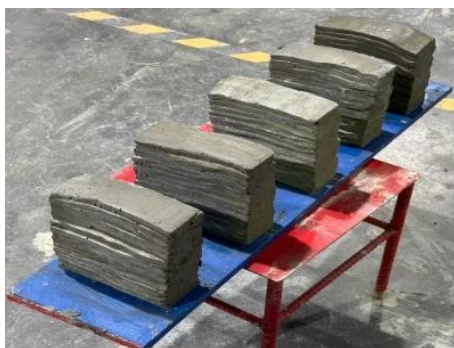
Fig. 5 3D Printed Concrete formwork
