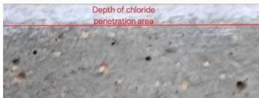
Fig. 12 Chloride penetration depth for wet-dry 15 cycles
