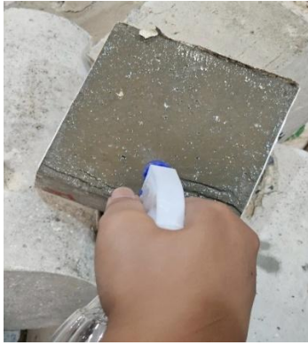
Fig. 11 Spraying Silver Nitrate Solution
