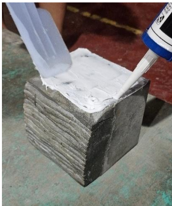
Fig. 8 Applying Epoxy to the concrete surfaces
