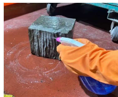
Fig. 7 Spraying Sika to concrete surface
