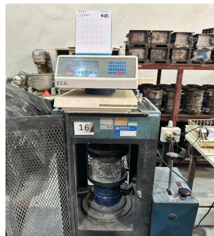
Fig. 10 Compressive strength test of Cubic Specimen
