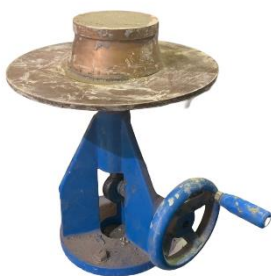
Fig. 5 Flowability test of mortar
