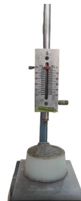
Fig. 6 Initial setting time test of mortar
