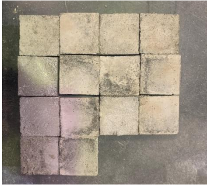
Fig. 4 50 x 50 x 50 mm specimens for compressive strength test
