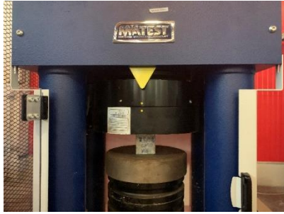
Fig. 7 Compressive strength test of mortar specimens
