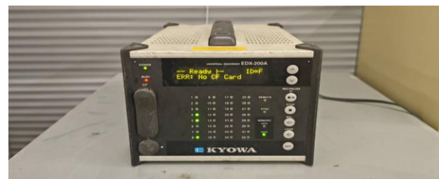
Fig. 5. Data logger applied during testing
