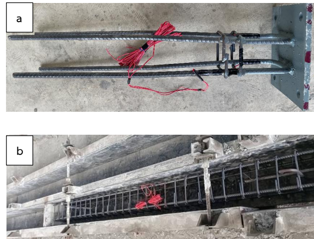
Fig. 4. Positions of strain gauges on (a) precast joint with bolt-plate connection and (b) conventional joint.
