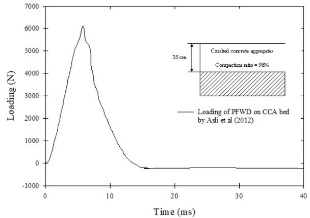
Fig. 5 Field FWD loading by Asli et al. [14]
