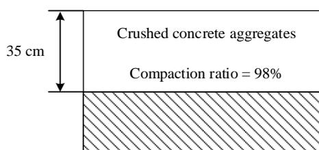
Fig. 4 Cross section of a concrete crushed aggregates soil system
