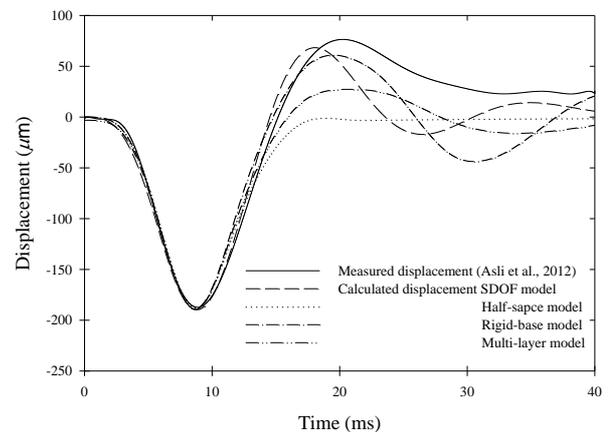
Fig. 6 Comparison of deflection profiles for concrete crushed aggregates (CCA) soil system from FWD field measurement and dynamic forward models
