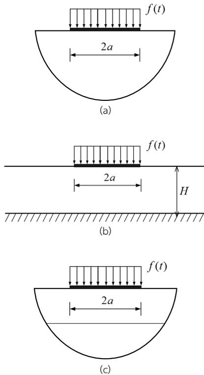
Fig. 3 Schematics of (a) half-space model, (b) rigid-base model and (c) multi-layered model
