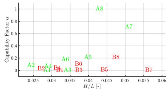
Fig. 14 Reduction of beach profile change offered by Flotilla as function of wave steepness ( $H/L$ ).
