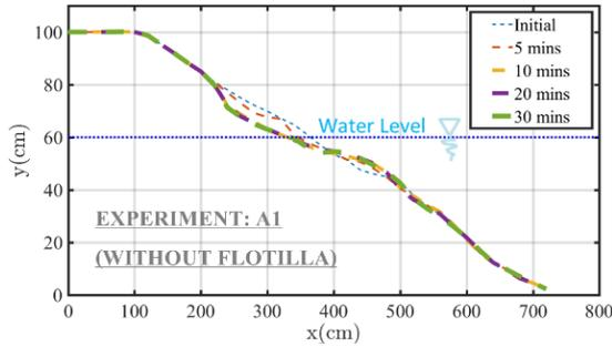
Fig. 7 Examples of evolving beach profiles in the first test (A1).
