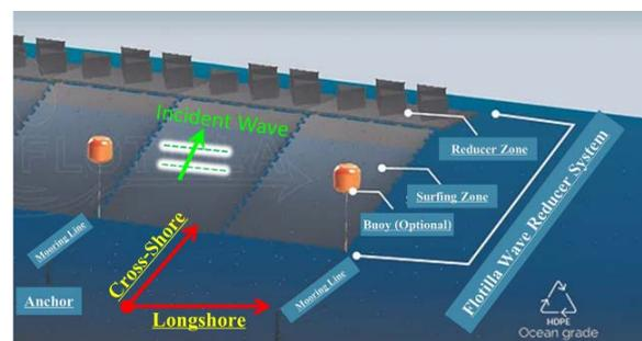
Fig. 1 An overview of Flotilla floating wave reducer system.
