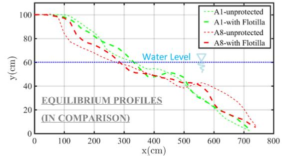
Fig. 9 Comparison of the profiles with/without Flotilla in Test Set A.
