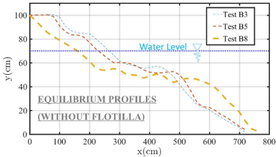
Fig. 8 Examples of equilibrium beach profiles observed in the experiment.
