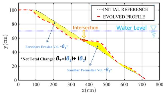
Fig. 11. Quantification of the net total change in beach profile evolution.
