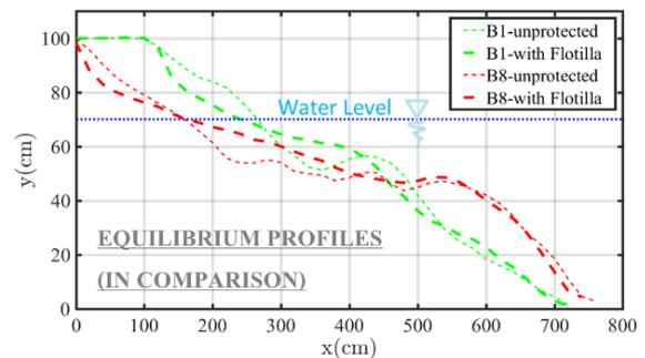
Fig. 10 Comparison of the profiles with/without Flotilla in Test Set B.
