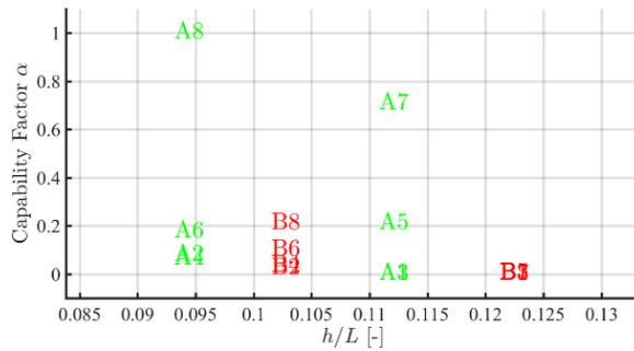
Fig. 15 Reduction of beach profile change offered by Flotilla as function of relative water depth ( $h/L$ ).
