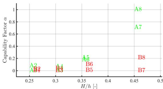
Fig. 13 Reduction of beach profile change offered by Flotilla as function of relative wave height ( $H/h$ ).
