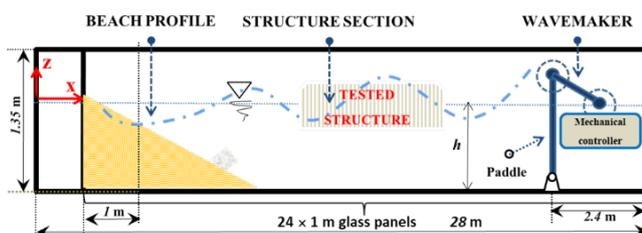
Fig. 4 Wave flume facility employed in the experimental study.
