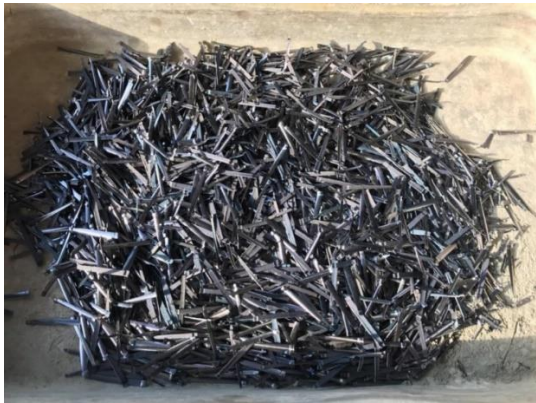
Fig. 2 Mill-cut steel fibers with hooked ends [3]
