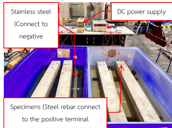
Fig. 3 Acceleration corrosion set up.
