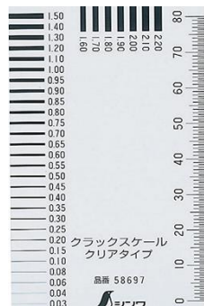
Fig. 5 Crack measurement tool
