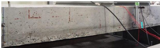
(a) At the first observable crack (at 136 kN)
