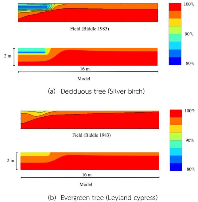
Figure 2 Degree of saturation during summer
