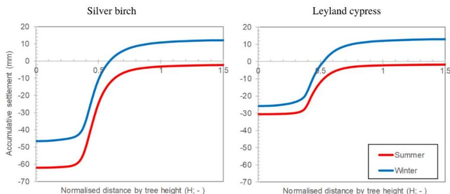
Figure 3 Plant effect on ground surface settlement during summer and winter
