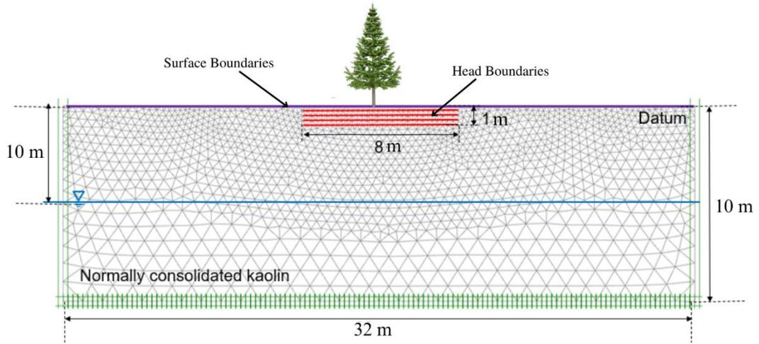
Figure 1 Model geometry
