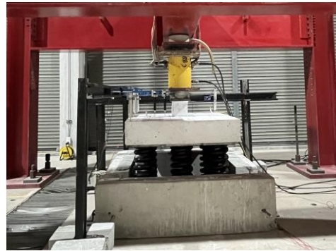
Fig. 4 Test setup on the elastic spring system
