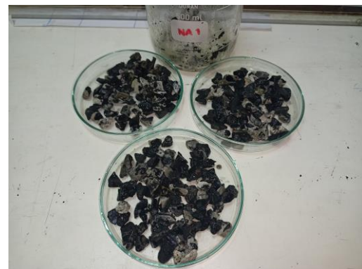
Fig. 2 The Rolling Bottle Test Result after 24 hours
