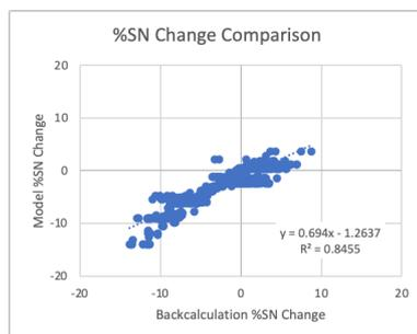
Fig. 8 Change of SN compare between BISAR and backcalculation from FWD test
