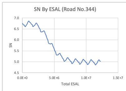
Fig. 7 SN pattern for CTB material
