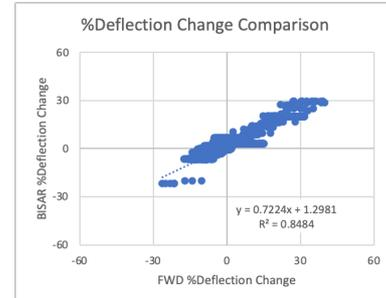
Fig. 5 Change of deflection compare between BISAR and FWD test
