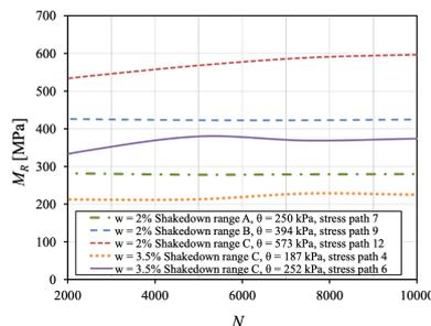
Fig. 2 Evolution of resilient modulus with number of load repetitions for different shakedown range [18]
