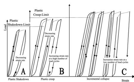
Fig. 1 Behavior of shakedown under repeated cyclic load in unbound materials [17]
