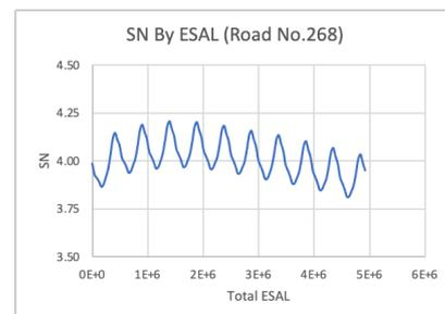
Fig. 6 SN pattern for unbound material
