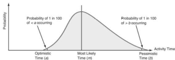
รูปที่1 Beta probability distribution PERT with three-time estimates[3]
