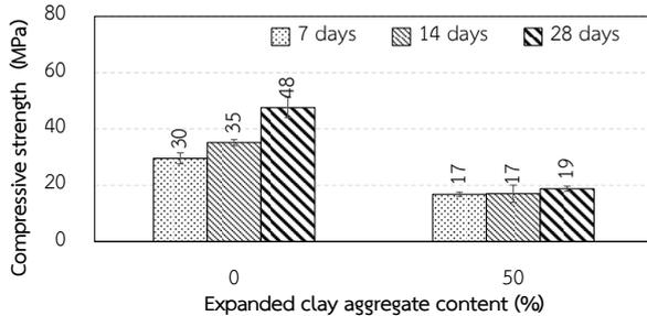
Fig. 4 Effect of expanded clay aggregate content on compressive strength
