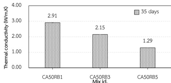
Fig. 8 Effect of biochar content with 50% of expanded clay aggregate on thermal conductivity
