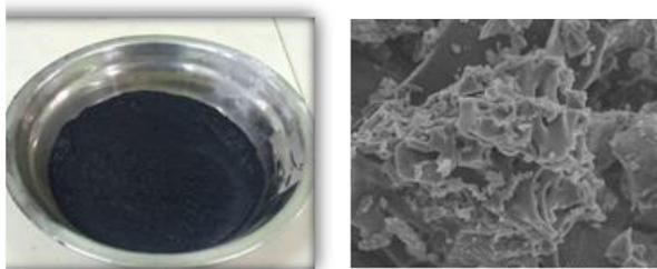
**Fig. 1** Biochar; (a) Powder and (b) SEM (x5000)
