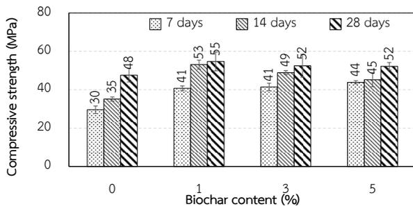
Fig. 3 Effect of biochar content on compressive strength
