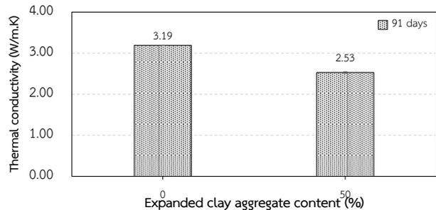
Fig. 7 Effect of expanded clay aggregate content on thermal conductivity
