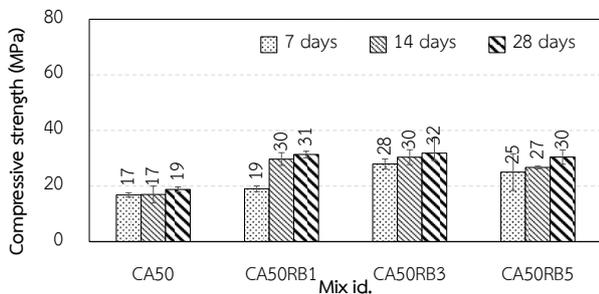
Fig. 5 Effect of biochar content with 50% of expanded clay aggregate replacement
