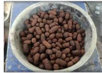
**Fig. 2** Expanded clay aggregate
