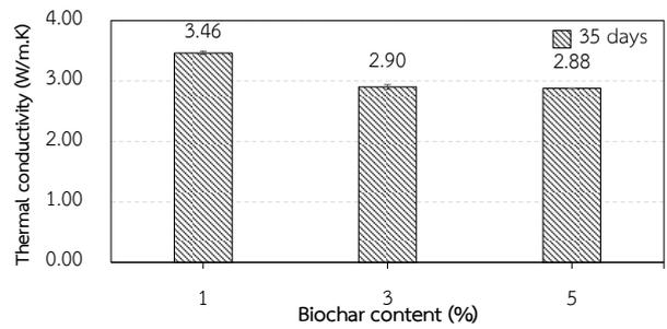
Fig. 6 Effect of biochar content on thermal conductivity
