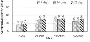
Fig. 5 Effect of biochar content with 50% of expanded clay aggregate replacement
