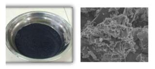
(a) (b) Fig. 1 Biochar; (a) Powder and (b) SEM (x5000)
