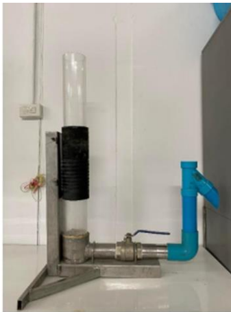
Figure 7 Permeability test equipment
