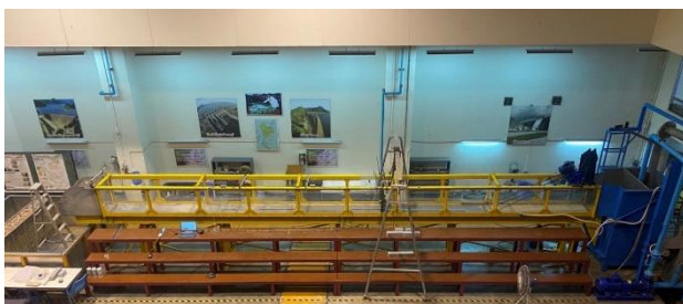
Figure 8 Hydraulic wave flume with the equipment setup for wave energy attenuation test
