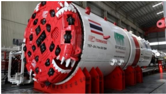
Fig. 2 The double shield TBM used in the TBM construction section https://www.rtco.co.th/portfolio
