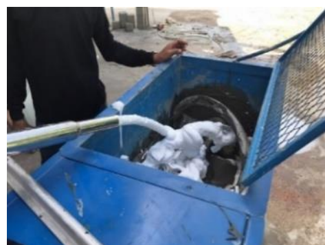
Fig 3. Adding foam agent into mortar
