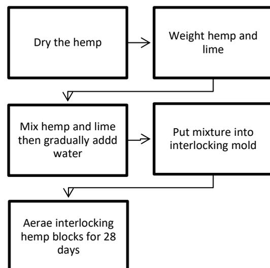
Figure 3 Hempcrete interlocking block processing
