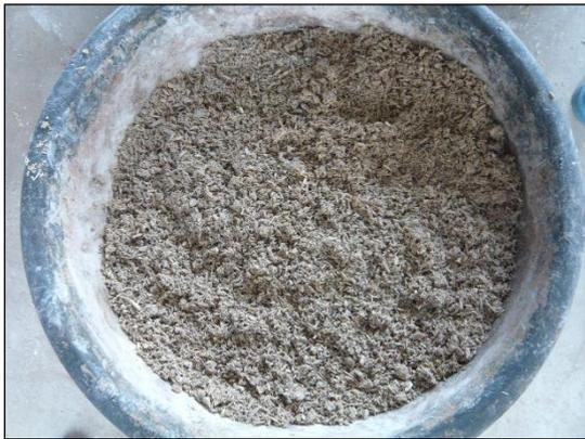
Figure 4 Hemp-lime mixture with appropriate moisture for molding.
