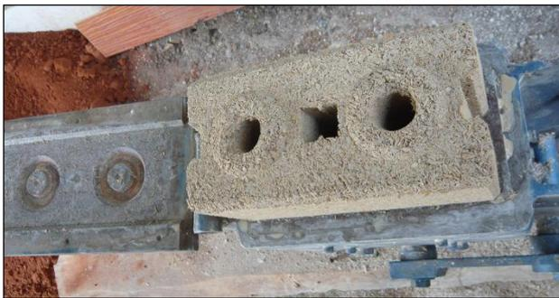
Figure 5 Interlocking hempcrete block molding
