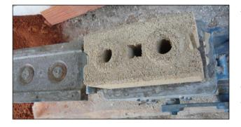
Figure 5 Interlocking hempcrete block molding
