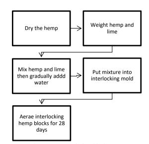
Figure 3 Hempcrete interlocking block processing
