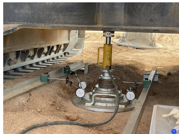
Fig. 8 Plate Load Test
