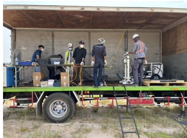
Fig. 7 Cone Penetration Test
