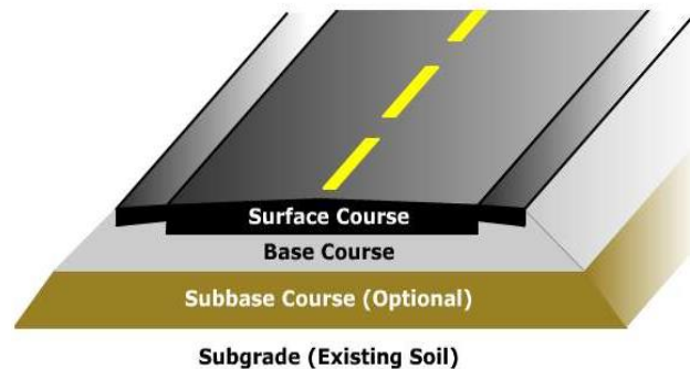
Fig. 2 A typical flexible pavement
