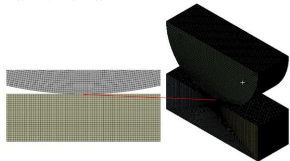
Fig. 1 Mapped mesh for finite element analysis
