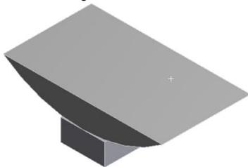
Fig. 2 Sub-modeling geometry in ANSYS®
