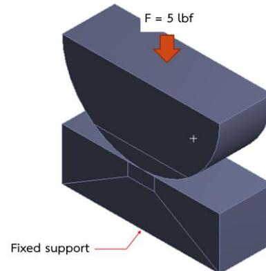
Fig. 3 Force and fixed support were applied in ANSYS®
