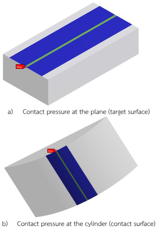
Fig. 4 Contact pressure result from ANSYS®
