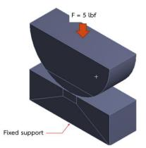
Fig. 3 Force and fixed support were applied in ANSYS® The data assumed for validation of Hertzian theory of a cylinder contact with a plane surface using finite element analysis was followed in Table 1.
