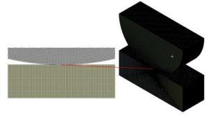
Fig. 1 Mapped mesh for finite element analysis 2.6 Sub modeling
