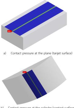
b) Contact pressure at the cylinder (contact surface)Fig. 4 Contact pressure result from ANSYS®
