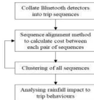
Fig. 2 Overview of the process using Sequence Alignment
