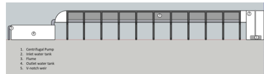
Figure 8 The open channel flume
