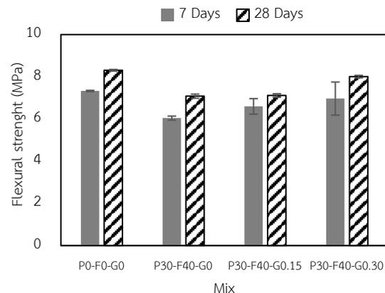
Figure 7. Flexural strength at curing age of 7 and 28 days
