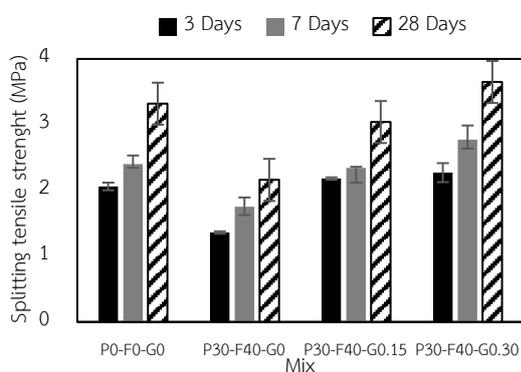
Figure 6. Splitting tensile strength at 3, 7, and 28 days
