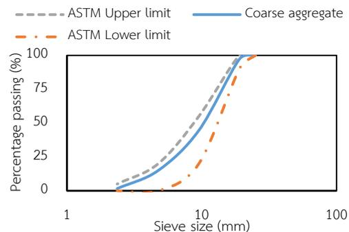
Figure 2. Particle size analysis of coarse aggregate
