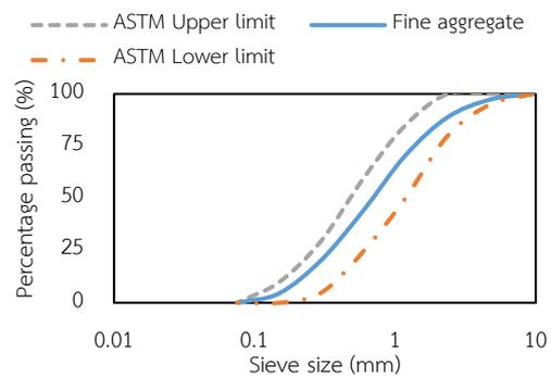
Figure 1. Particle size analysis of fine aggregate
