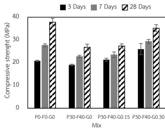
Figure 5. Compressive strength at 3, 7, and 28 days.
