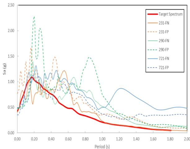
Fig. 6 Response spectra of ground motions used in this study.
