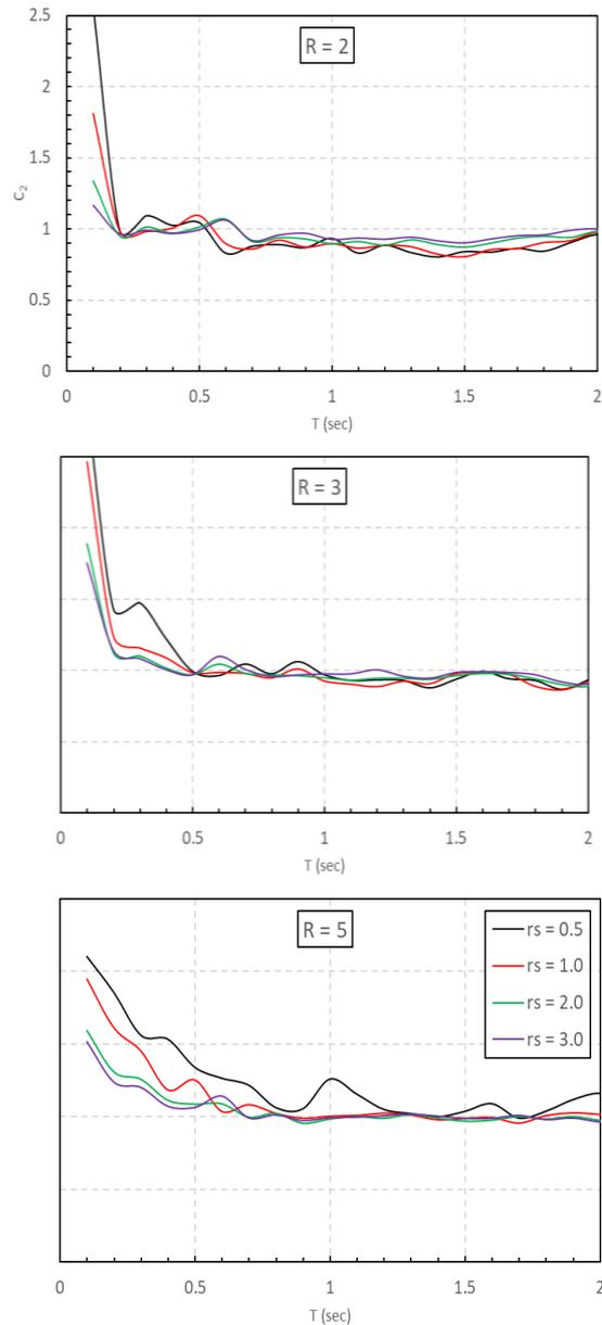
Fig. 3 Values of  $C_2$  factor for different strength ratios compared with those from FEMA440 (Khampanit and Leelatviwat 2015).
