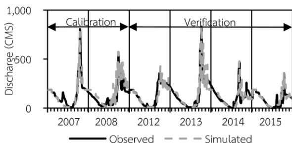
Fig. 4 Calibration and validation of Inflow discharge results at hydrological station (S.39) from HEC-HMS model
