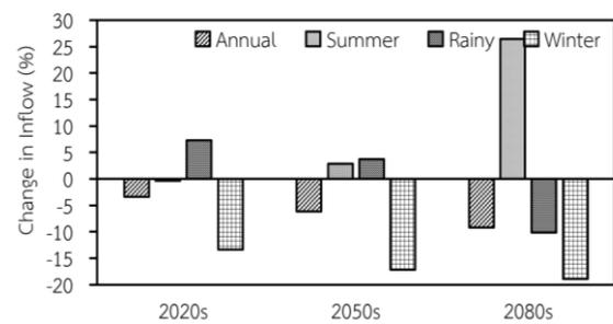
Fig. 6 Percentage changing in inflow discharge to Pasak Jolasid Dam on 2020s, 2050s and 2080s
