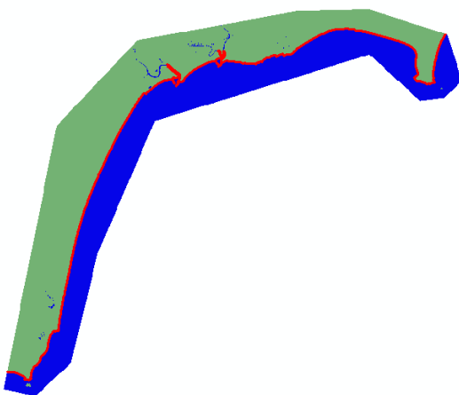
Fig. 6 Determine shoreline by smoothing NDWI contour line case of 03 March 2020
