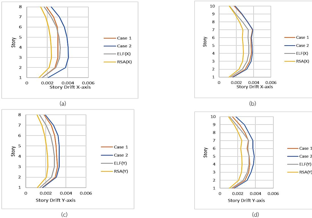
Fig. 6 Story drift ratio calculated from ELF, RSA and LTHA (a) 8story(X-X), (b) 10story(X-X), (c) 8story(Y-Y) and (d) 10story(Y-Y)
