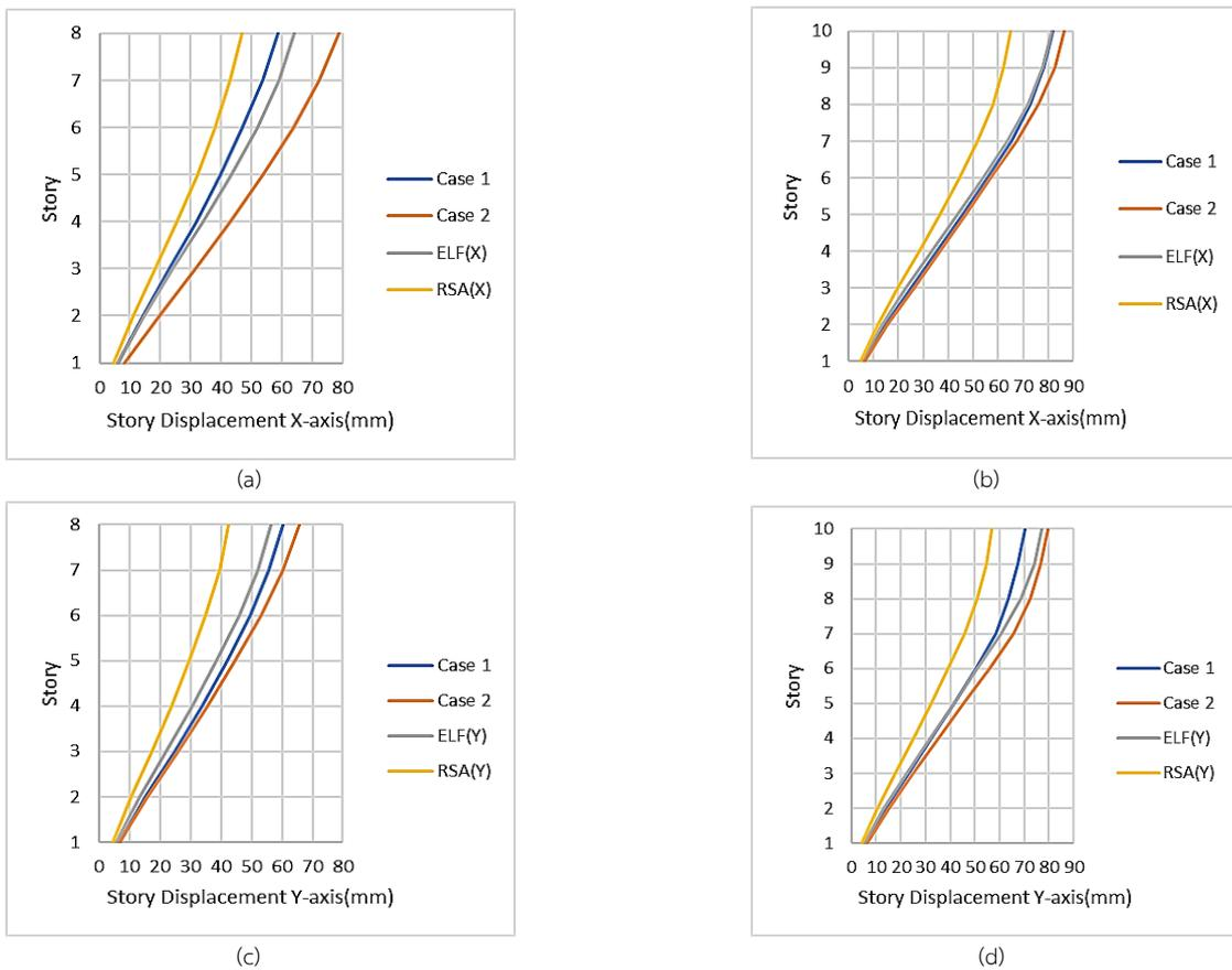
Fig. 7 Story displacement calculated from ELF, RSA and LTHA (a) 8story(X-X), (b) 10story(X-X), (c) 8story(Y-Y) and (d) 10story(Y-Y)
