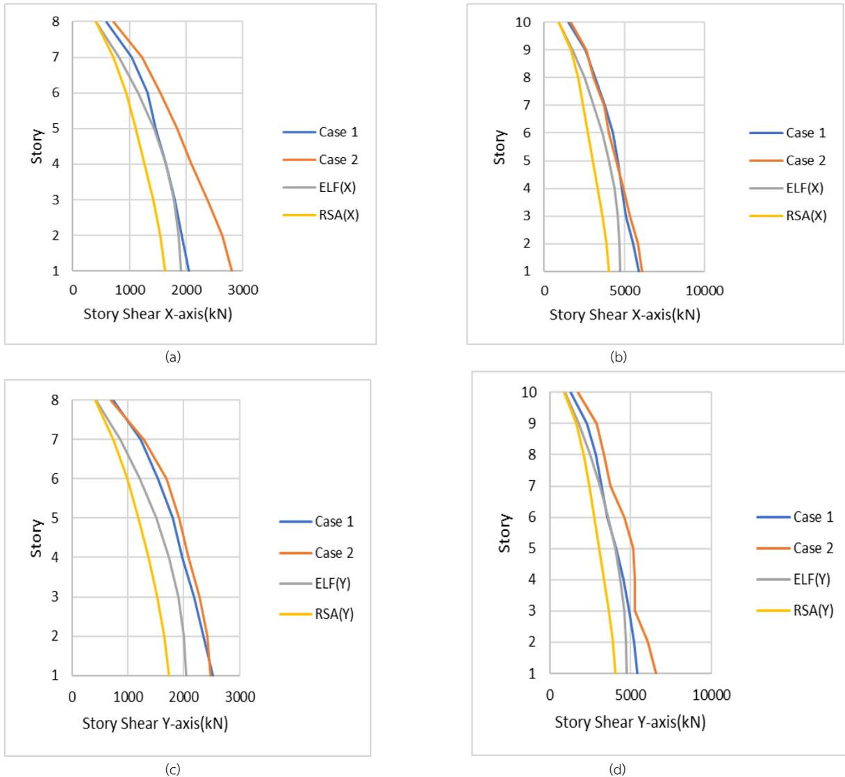
Fig. 8 Story shear calculated from ELF, RSA and LTHA (a) 8story(X-X), (b) 10story(X-X), (c) 8story(Y-Y) and (d) 10story(Y-Y)
