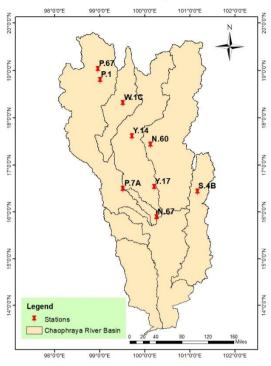
Fig. 1 Location of key stations in Chao Phraya River Basin Key stations are selected based on having regular long-term maintenance to generate representative series of river system and locations free of backwater effects from any existing, ongoing or future. The generated datasets; observed and forecasted discharge from HII's flood forecasting system are collected and used in this study.
