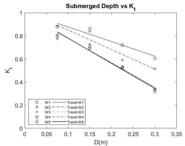
Fig.8 Relation of wave transmission coefficient and submerged depth
