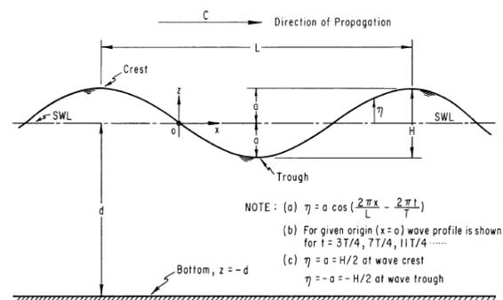
Fig.2 Definition of Wave Parameters [5]
