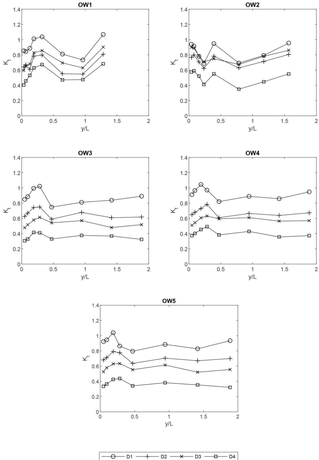
Fig.7 The wave transmission coefficient and the ratio of distance in cross-shore direction to wave length ( $y/L$ )
