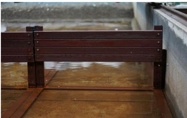
(b) The layer of artificial partial breakwater
