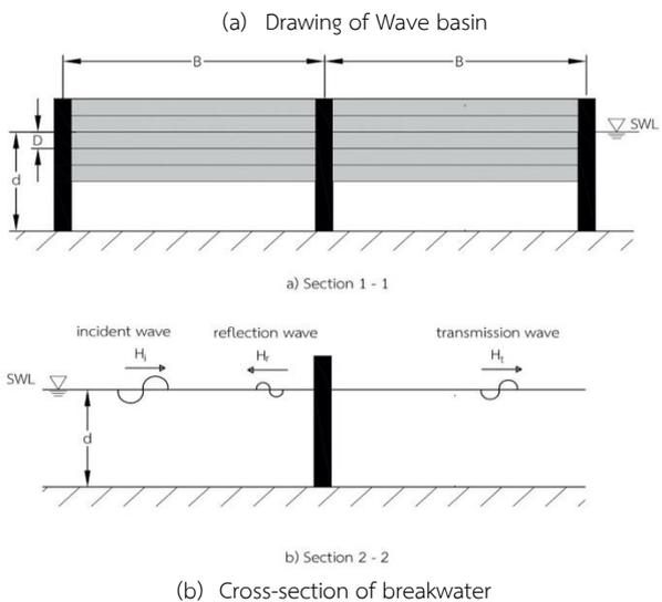
**Fig.3** Wave basin and location of Breakwater
