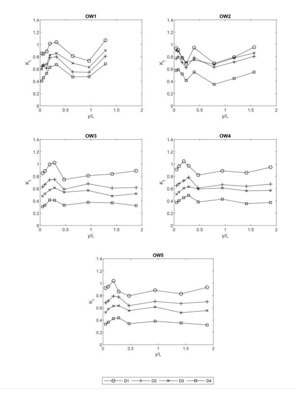
Fig.7 The wave transmission coefficient and the ratio of distance in cross-shore direction to wave length (y/L)
