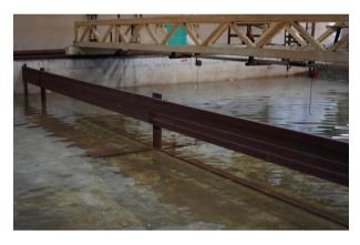
(a) The construction of artificial partial breakwater
