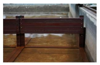
(b) The layer of artificial partial breakwater
