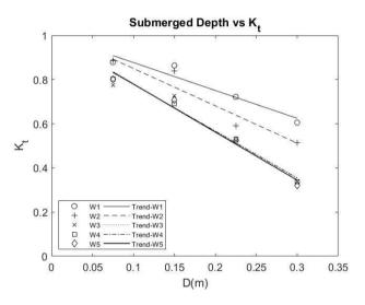
Fig.8 Relation of wave transmission coefficient and submerged depth
