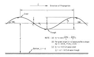
Fig.2 Definition of Wave Parameters [5]
