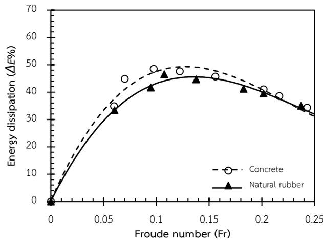
Fig. 16 The relationship between energy dissipation and discharge of natural rubber and concrete tetrapods with 63.77% of porosity
