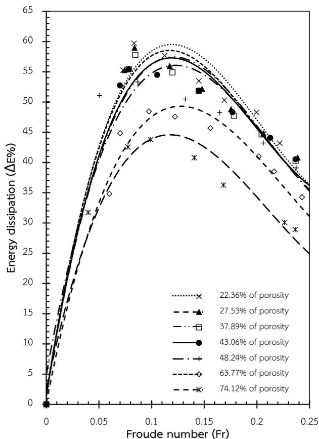
Fig. 19 The comparison of energy dissipation by using concrete tetrapods with different porosities
