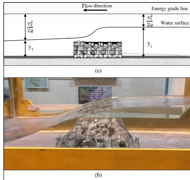
Fig. 10 The energy dissipation (a) sketch (b) real experiment in laboratory
