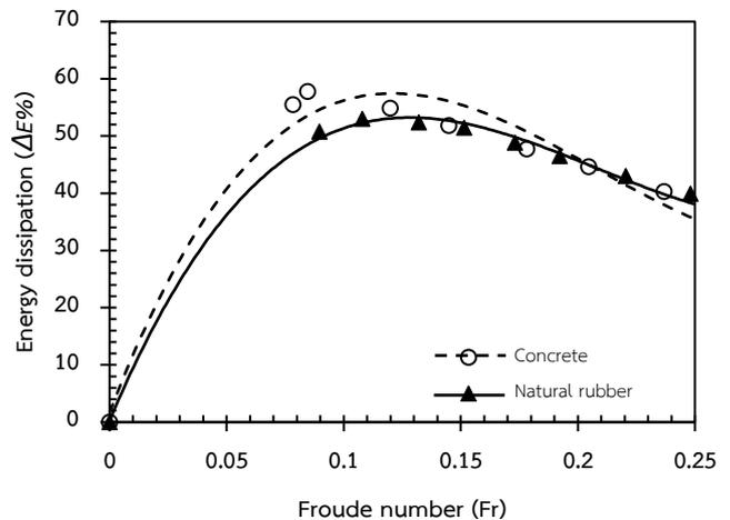
Fig. 13 The relationship between energy dissipation and discharge of natural rubber and concrete tetrapods with 37.89% of porosity
