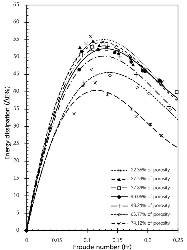
Fig. 18 The comparison of energy dissipation by using natural rubber tetrapods with different porosities
