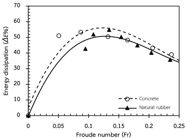
Fig. 15 The relationship between energy dissipation and discharge of natural rubber and concrete tetrapods with 48.24% of porosity
