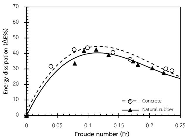
Fig. 17 The relationship between energy dissipation and discharge of natural rubber and concrete tetrapods with 74.12% of porosity
