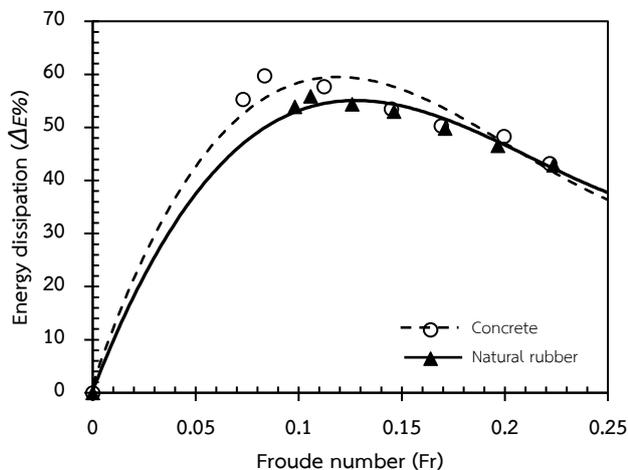
Fig. 11 The relationship between energy dissipation and discharge of natural rubber and concrete tetrapods with 22.36% of porosity.
