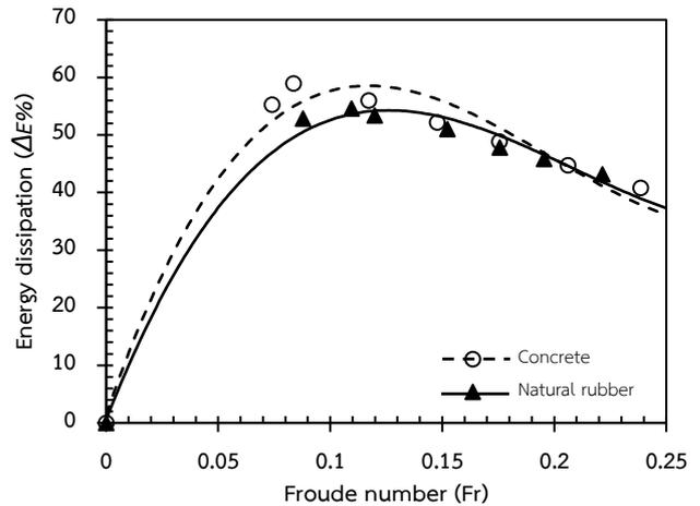
Fig. 12 The relationship between energy dissipation and discharge of natural rubber and concrete tetrapods with 27.53% of porosity
