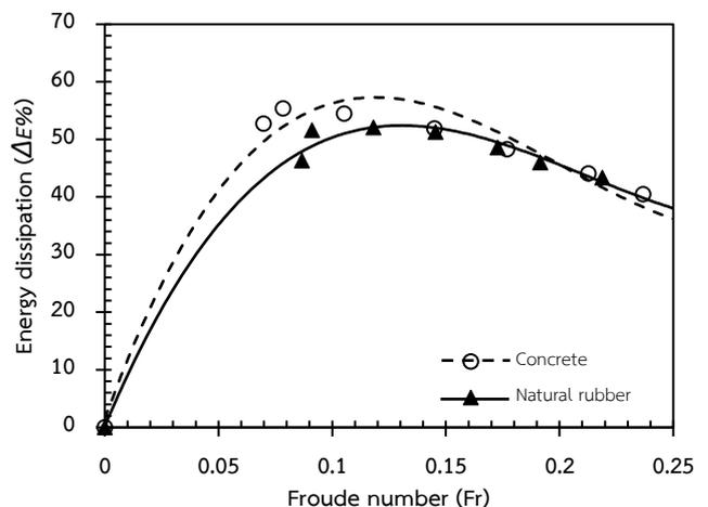
Fig. 14 The relationship between energy dissipation and discharge of natural rubber and concrete tetrapods with 43.06% of porosity
