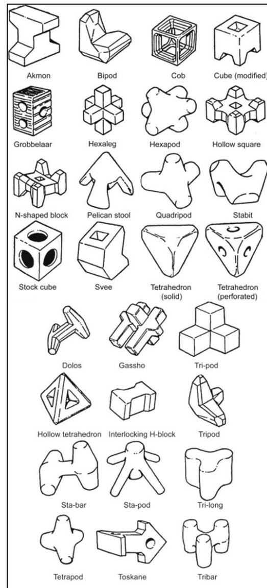
Fig. 2 Shapes of concrete armor block [3]
