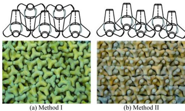
Fig. 3 Tetrapod placement methods [4]
