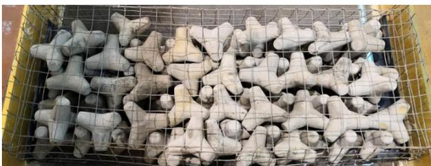
Fig. 9 Concrete artificial tetrapod placement
