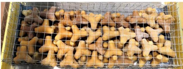
Fig. 8 Natural rubber artificial tetrapod placement
