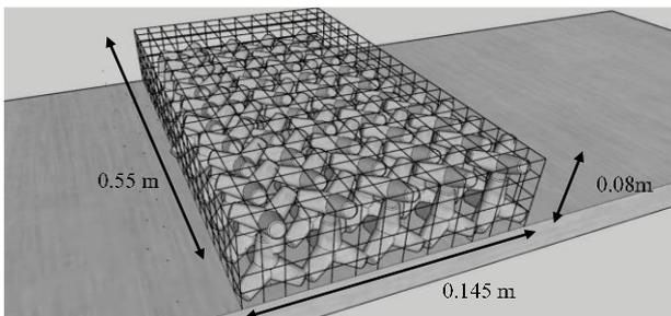
Fig.7 Tetrapod model setup
