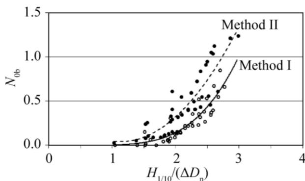
Fig 4. Stability of tetrapod placement methods I and II [4]
