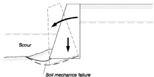
Fig. 8 Seaward overturning and settlement of gravity wall [4]
