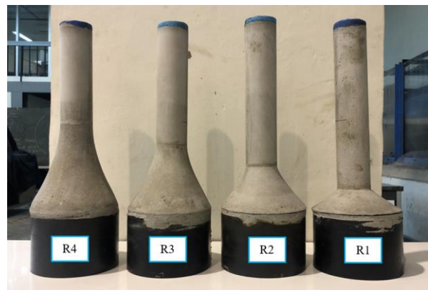
Fig. 12 The 4 configuration models of pier with based ramp
