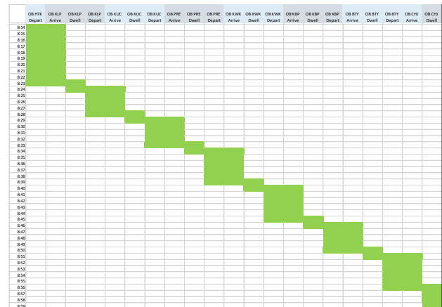
Fig. 5 Blocking time diagram of train #283, before compression.
