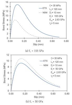
Fig. 7 Effects of bond stress-slip responses in each strengthening
